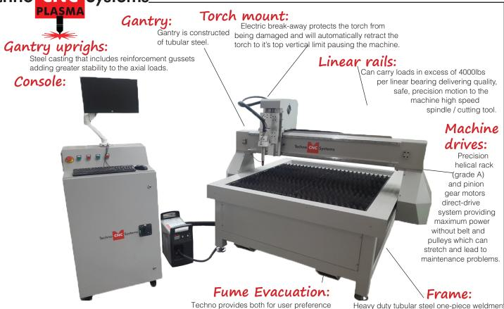
Frame: Techno HD-II Series Frame is a tubular steel weldment that is precision machined, and stress relieved so that it remains true over the life of the machine. Weight 3000lbs.
